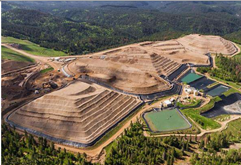
Fig. 1. Mine OB dump with benches
